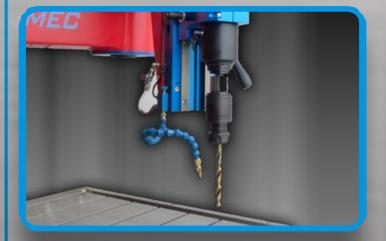
WITH THIS SYSTEM IS POSSIBLE TO ENSURE A CORRECT NEBULIZATION'S TOOL.
